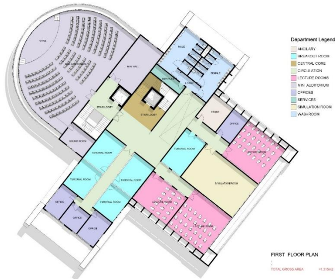
Figure 2-5: Multi-purpose Educational Complex First floor layout
