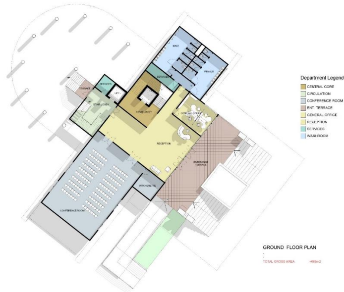
Figure 2-4: Multi-purpose Educational Complex Ground floor layout
